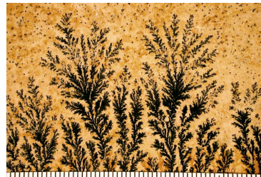
Manganese deposition on a limestone
